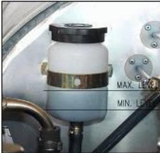
INSPECT – oil, quantity (between MIN and MAX marks), leakages. The oil level should be at least in the middle between marks when planning a long term operation.
