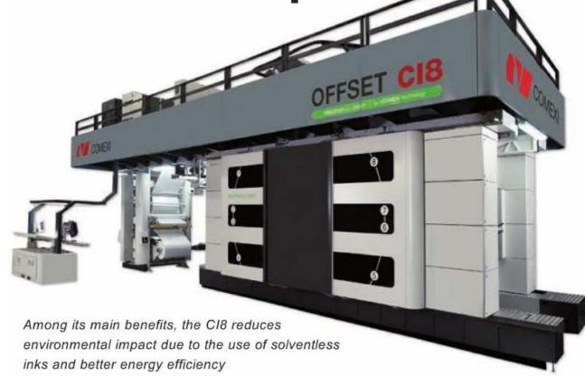
drum it combines the advantages of both offset variable print length and flexo central impression drum printing in one press for flexible packaging and labels. This combination overcomes the issues found with conventional in-line offset machines because it can easily print thinner and more elastic materials including OPP, PET and PE.
