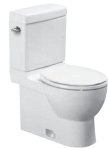
TWIST 5C11 01 Round-front 12" rough-in 1.28 gpf, siphonic jet 5D07 U1 Tank 9M08 U1 seat & cover with quick release & soft-closing hinges
