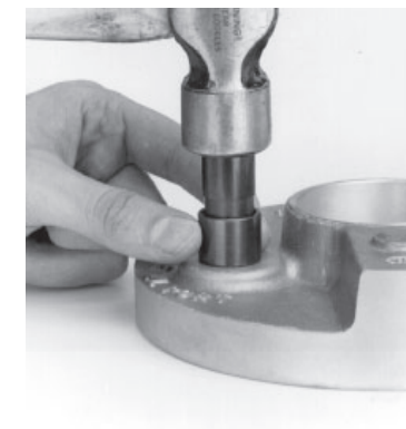
4. Push in the keys by hitting on the fitting tool
