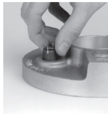
3. Screw the Clav-Sert insert into the housing
